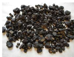
Treated RA 110°C → disintegration
